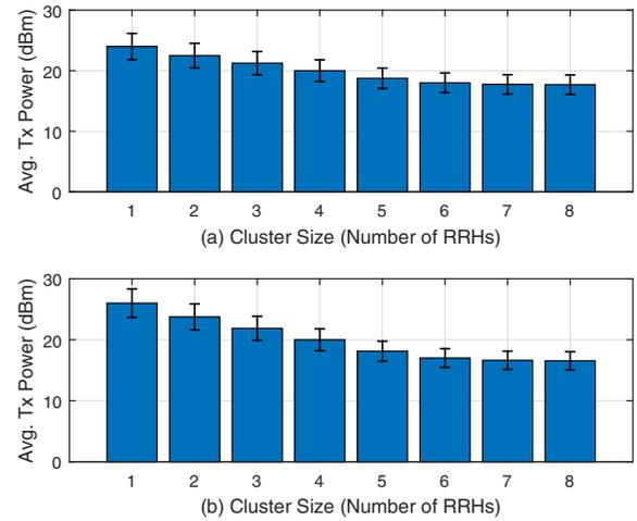
Fig. 5. Average Per-RRH Transmit Power versus Cluster Size with  $\epsilon = 0.1$ ,  $\rho_u = 0.1$ ,  $\forall u$  and average per-user delay being 20 packets; (a) Uniform user distribution and (b) Non-uniform user distribution.
