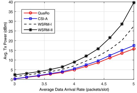
Fig. 4. Average per-RRH transmit power versus average data arrival rate with  $\epsilon = 0.1$ ,  $\rho_u = 0.1$ ,  $\forall u$  and average per-user delay being 20 packets.
