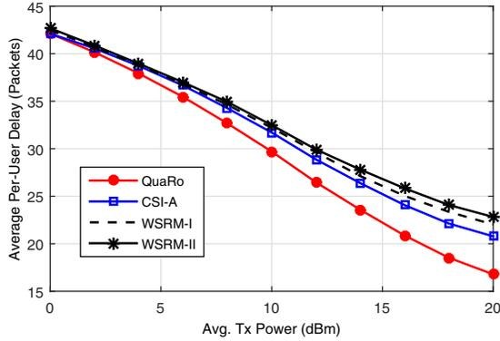
Fig. 3. Average per-user delay versus average per-RRH transmit power with  $\epsilon = 0.1$ ,  $\rho_u = 0.1$  and  $\lambda_u = 5$  packets/slot,  $\forall u$ .
