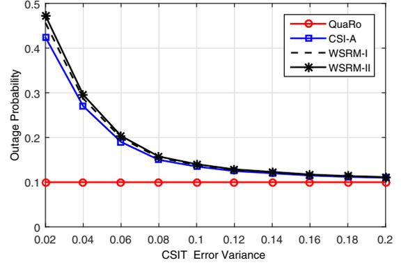
Fig. 2. Outage probability versus CSIT error variance with scheduled rate  $R_u = 1$  bit/s/Hz,  $\forall u$ .
