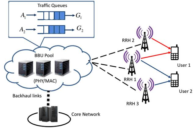
Fig. 1. Cloud Radio Access Network Architecture.
