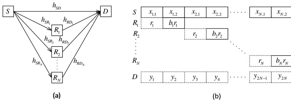
Fig. 1. (a) The half-duplex NAF multi-relay system. (b) The frame structure of the NAF multi-relay protocol; the solid boxes denote the transmitted signals and the dashed boxes denote the received signals.
