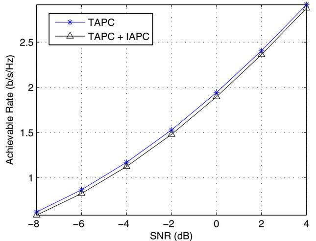
Fig. 3. The achievable rate of the OAF system with CSI under TAPC and under both TAPC and IAPC.
