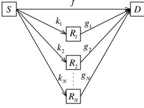
Fig. 1. The half-duplex multiple-relay OAF system.
