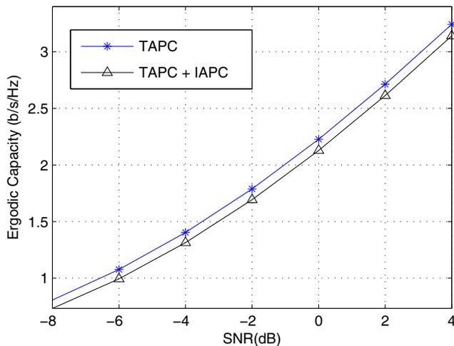
Fig. 5. The ergodic capacities of the OAF system under TAPC and under both the TAPC and IAPC.
