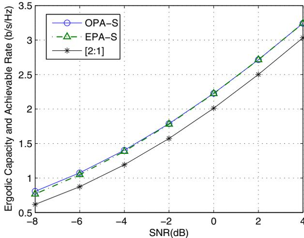
Fig. 4. The ergodic capacity and achievable rate of the OAF systems with different power allocation schemes at the source under the TAPC.
