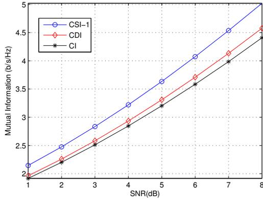
Fig. 3. The MI of different NAF systems over a symmetric channel with  $d_{SD} = d_{SR1} = d_{SR2} = d_{RD1} = d_{RD2} = 1$ .
