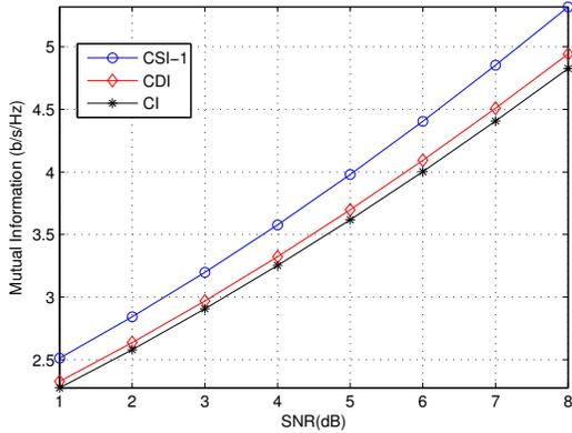
Fig. 4. The MI of different NAF systems over an asymmetric channel with  $d_{SD} = 1, d_{SR1} = d_{RD1} = 1.5, d_{SR2} = d_{RD2} = 0.5$ .
