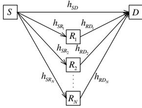
Fig. 1. The half-duplex multiple-relay NAF system.
