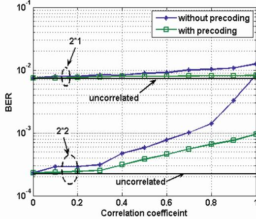
Figure 6. BER of the STBC Multiuser CDMA system in correlated channel, against correlation coefficient value considering the effect of precoding.
