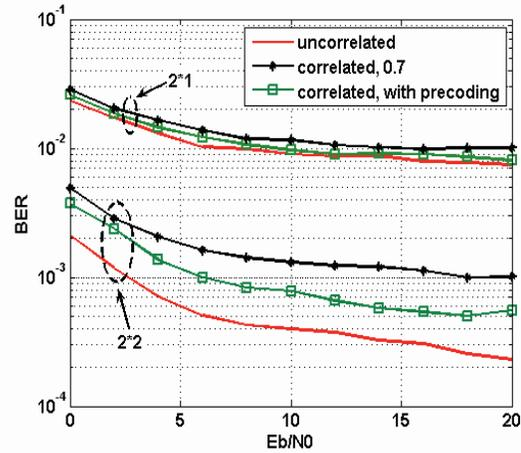
Figure 4. BER of the STBC Multiuser CDMA system in correlated channel considering the effect of precoding.
