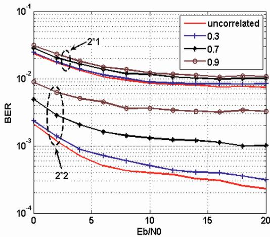
Figure 3. BER of the STBC Multiuser CDMA system in correlated channel considering the effect of correlation coefficient value.
