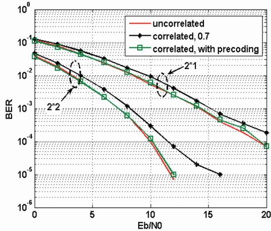
Figure 2. BER of the STBC single user system in correlated channel considering the effect of precoding.
