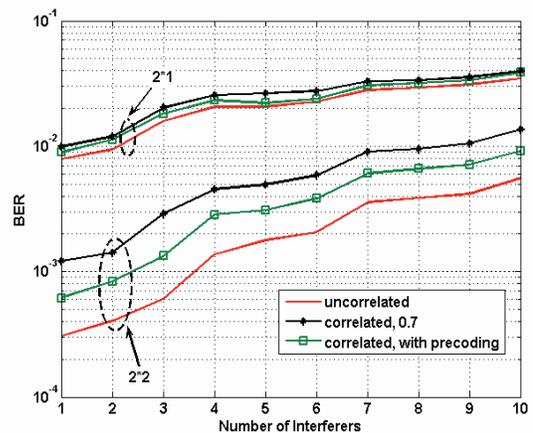
Figure 5. BER of the STBC Multiuser CDMA system in correlated channel considering the effect of number of interfering users.
